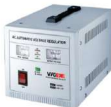
MODEL NO: MVR-1500VA Input: 150-270V~ 50Hz Output:230V~ 50Hz Power:1500VA Technology: Analog Circuit + Meter Display + Servo Motor High Voltage Protection Low Voltage Protection Overload Protection High Temperature Protection
