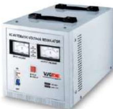
MODEL NO: MVR-3000VA Input: 150-270V~ 50Hz Output:230V~ 50Hz Power:3000VA Technology: Digital Circuit +Meter Display + Servo Motor High Voltage Protection Low Voltage Protection Overload Protection High Temperature Protection
