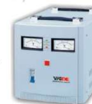
MODEL NO: TVR-8000VA Input: 150-270V~ 50/60Hz Output:230V~ 50/60Hz Power:8000VA Technology: Meter Display + C.R.G.O Transformer High Voltage Protection Low Voltage Protection Overload Protection High Temperature Protection
