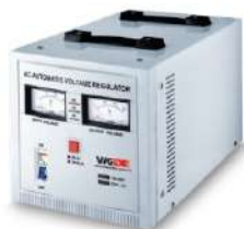
MODEL NO: MVR-3000VA Input: 150-270V~ 50Hz Output:230V~ 50Hz Power:3000VA Technology: Digital Circuit +Meter Display + Servo Motor High Voltage Protection Low Voltage Protection Overload Protection High Temperature Protection
