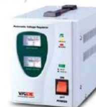
MODEL NO: SVR-1000VA Input: 150-270V~ 50Hz Output:230V~ 50Hz Power:1000VA Technology: Analog circuit+ meter display High Voltage Protection Low Voltage Protection Overload Protection High Temperature Protection
